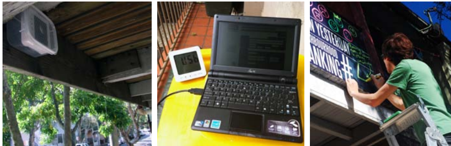
Figure 3. Left: Hidden storage of a separate electricity monitor allowing uninterrupted access to the data. Center: Netbook and electricity monitor used for downloading and updating displays. Right: The manual update of the daily neighborhood ranking using a ladder.
